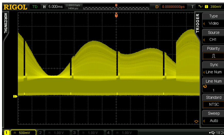
Figure 3-11 NTSC Video Signal
