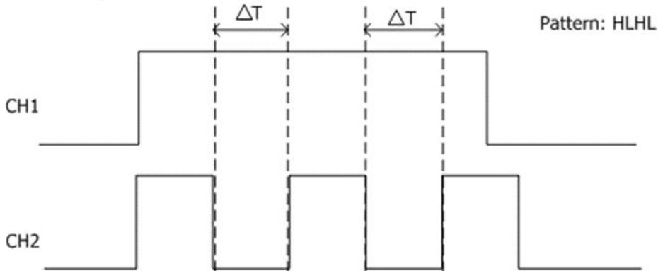
Figure 5-7 Duration Trigger
