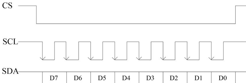
Figure 5- 15 Sequential Chart of SPI Bus
