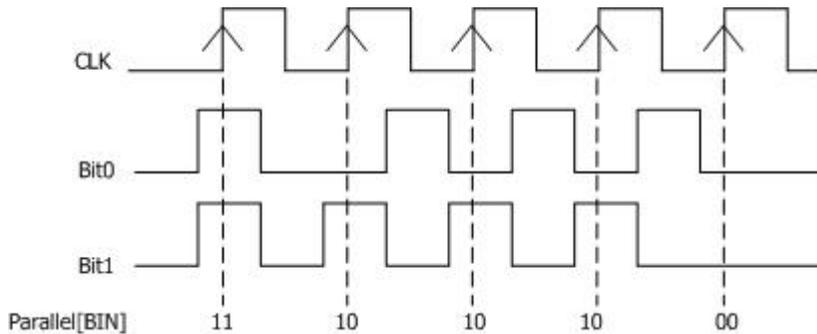
Figure 7- 1 Parallel Decoding
