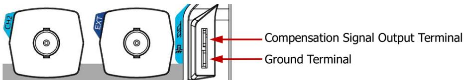
Figure 1-6 To Use the Compensation Signal
