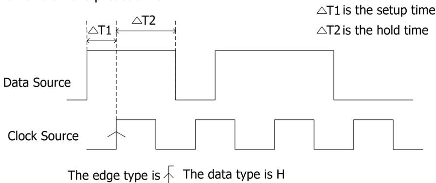
Figure 5- 11 Setup/Hold Trigger
