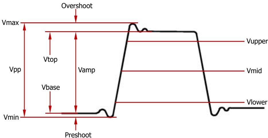
Figure 6-5 Voltage Parameters
