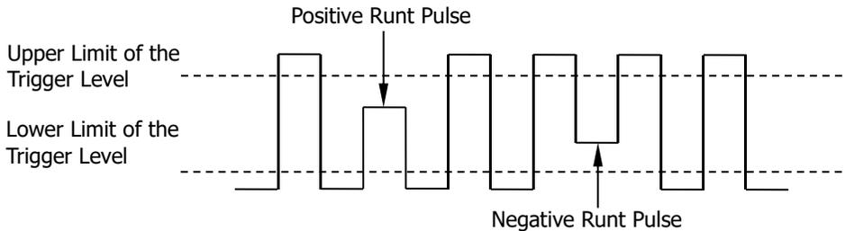
Figure 5-9 Runt Trigger
