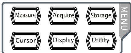
**Measure**: press this key to open the measurement setting menu. You can set the measurement source, turn on or off the frequency counter, all measure, statistic function and etc. Press **MENU** at the left of the screen to open the measurement menus of 37 waveform parameters. Then, press down the corresponding menu softkey to quickly realize one-key measurement and the measurement result will be displayed at the bottom of the screen.
