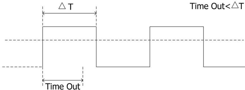
Figure 5-8 TimeOut Trigger
