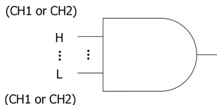
Figure 5-6 Pattern Trigger
