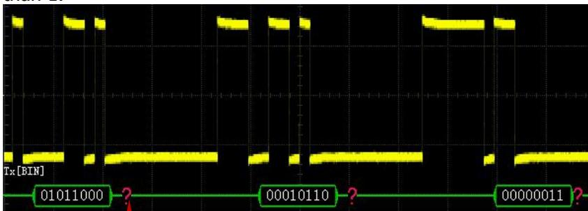
The stop bit is less than 1
