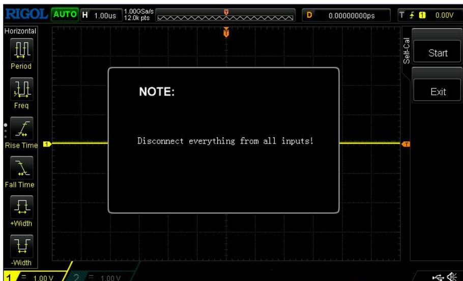
Figure 13-2 Self-calibration Interface
