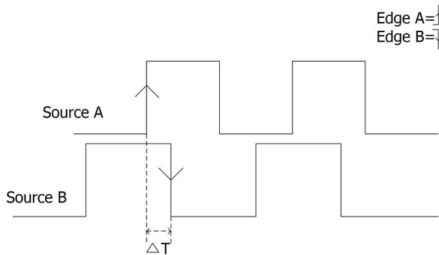
Figure 5-10 Delay Trigger
