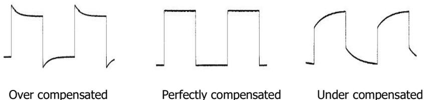
Figure 1-8 Probe Compensation
