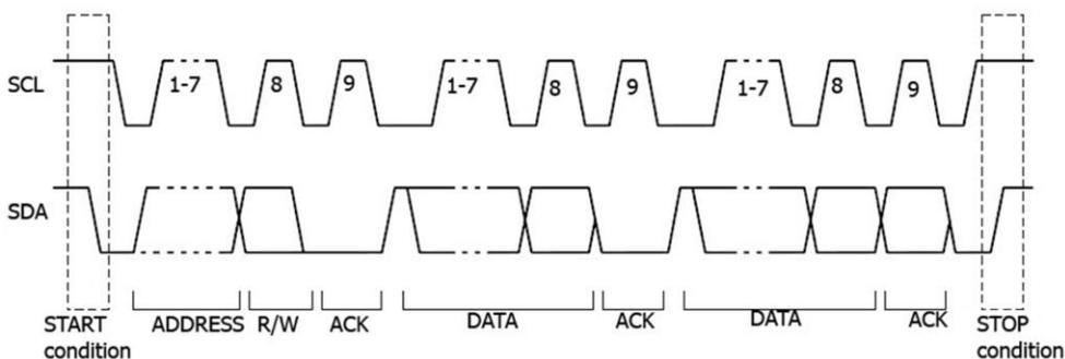
Figure 5- 14 Schematic Diagram of I2C Protocol
