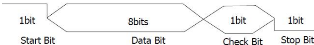
Figure 5- 13 Schematic Diagram of RS232 Protocol
