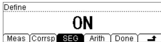
Figure 2-47 On/Off section interface of Arithmetic
