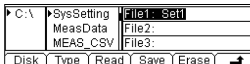
Figure 3-30 Configuration save interface
