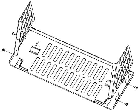
2. Install the front panel: let the screw holes fit well together and fix them with six M4 screws.
